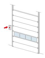
With this control system an electric motor actuates the shaft (using cable drums and balance springs). The rotation of the shaft moves the door up or down. The motor is not supposed to absorb an incorrect balance
