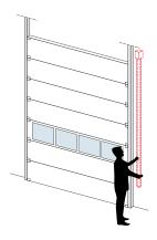
With the manual chain hoist model the shaft (using cable drums and balance springs) are manually driven. A unit with a circular chain has been installed at the end of the shaft. This control chain hangs in a loop next to the door. Depending on the direction of movement of the chain, the door panel moves up or down. To open/close using a manual chain hoist:
